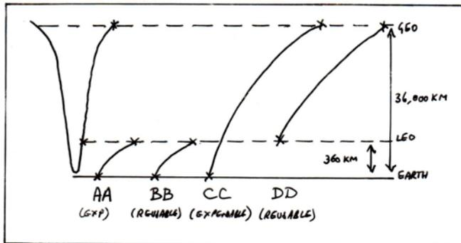
Fig App 1 Comparison cases for various ways of getting crews or cargo out of Earth’s gravity well and up to GEO
