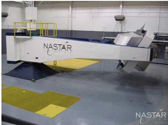
Fig 1 Commercial high-g training centrifuge at NASTAR center
