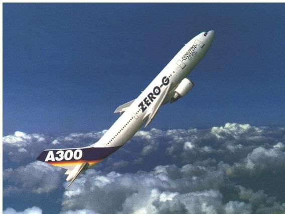
Fig 2. Zero-g experience is available via parabolic flight trajectory.
